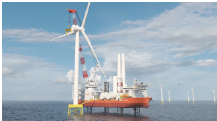
Figure 15. Illustration of a turbine installation vessel, jack up vessel
